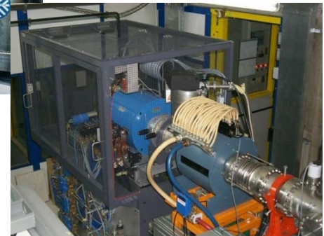
Superconducting ECR source SERSE
