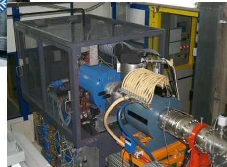
Superconducting ECR source SERSE
