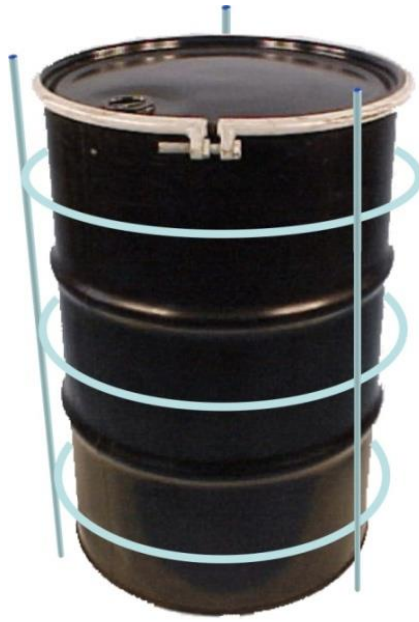
Fig.6 A possible arrangement of the fibers around a radwaste drum
