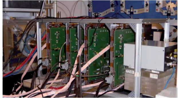
Figure 2: Photograph of the pCR system, composed by four Si x -y planes and a YAG:Ce calorimeter with front-end electronics, installed at CATANA beam in LNS INFN.
