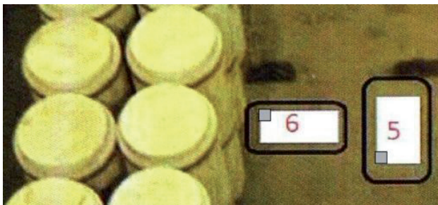
Fig. 4. The positions P5 and P6 of the pushcart with respect to the drums. The grey square indicates the position of the geiger counter on the cart.
