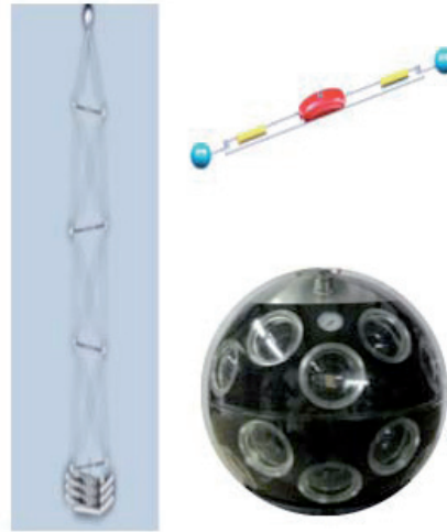
Figure 8: Sketch of the KM3NeT PPM; the Detection Unit, the storey (bar) and a photo of the DOM prototype.
