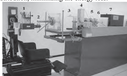
Figure 1: View of the CATANA beam line: 1. Treatment chair for patient immobilization; 2. Final collimator; 3. Positioning laser; 4. Light field simulator; 5. Monitor chambers; 6. Intermediate collimator; 7. Box for the location of modulator wheel and range shifter.
