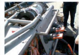
Figure 2: The Capo Passero deep-sea Junction Box, successfully deployed in November 2009. A detail showing the three ROV operable connectors is shown on the right.
