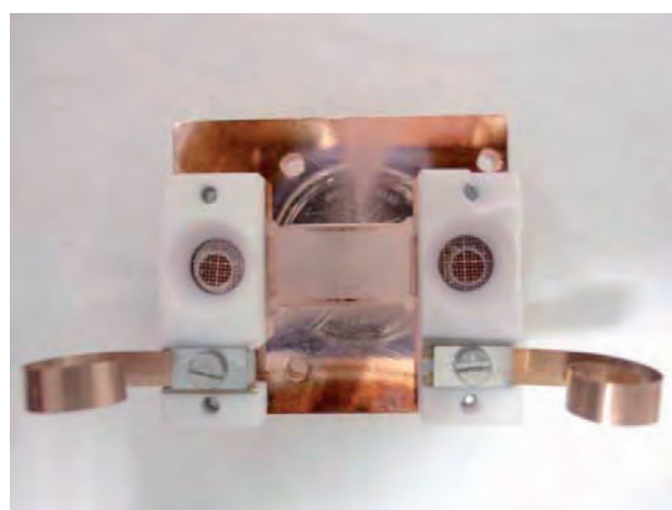
Figure 2: The copper support, holding two CNTs electron guns.
