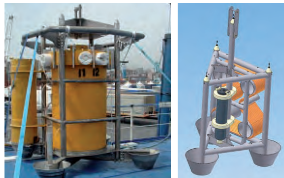
Figure 6: Left- The NEMO Junction Box. Right- Design of the deep sea frame holding the LIDO TSS station.
