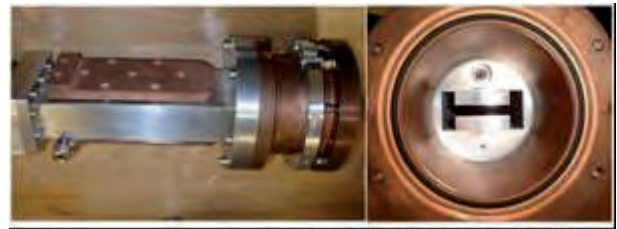
Figure 3 : A photo of the matching transformer (left) coupled to the plasma chamber (right) and its inner view.
