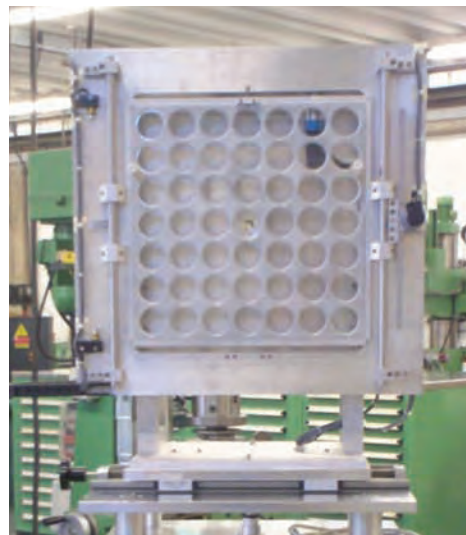
Figure 1: Photo of the experimental set-up. In the picture, the sample charger that allows to holder the Petri dishes is shown
