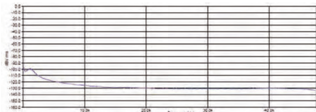
Figure 5: Electronics noise spectrum measured for a channel of the LIDO TSN acoustic data chain.
