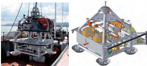
Figure 3: Left- The SN1 Station hanged to the MODUS deep sea shuttle before the deployment (2005). Right- Mechanical structure of the LIDO TSN station.
