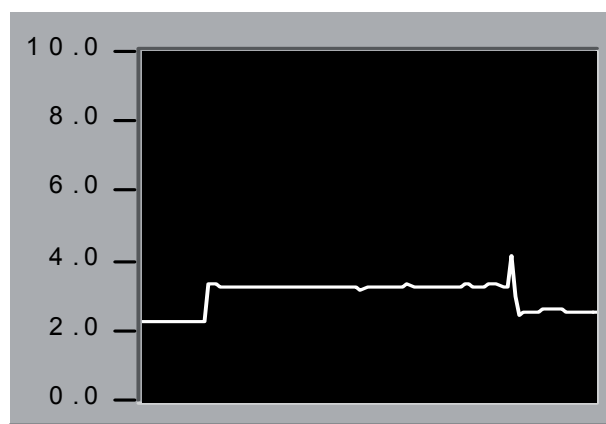
Figure 4: Trend of the \text{Kr}^{11+} current (in \mu\text{A} ) during the switching on-off of CNTs emission, in a time window of 30 seconds (an afterglow peak is evident at the switching off).
