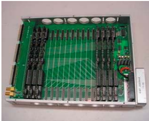
Figure 1: 16 channel NIM module including Fast amplifier, CFD's and Energy amplifier.
