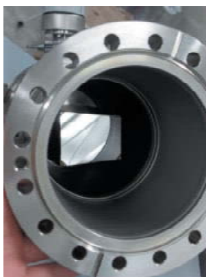
Fig.2: View of the \Delta E -E telescope used to identify the fragmentation products.
