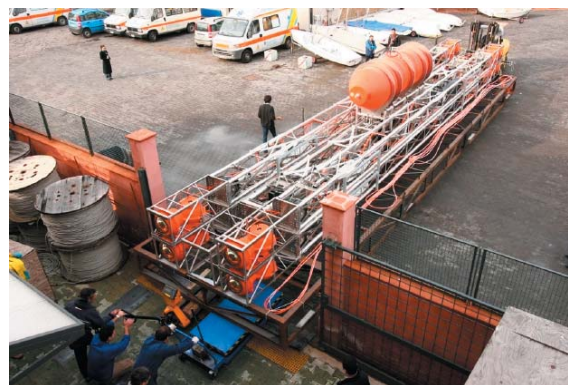
Fig. 4 - The mini-tower with the 4 floors packed at the exit from the LNS shore station.
