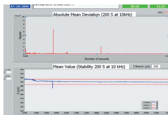
Fig. 2 – A plot taken during reliability measurements (the red lines show the acceptable limits).
