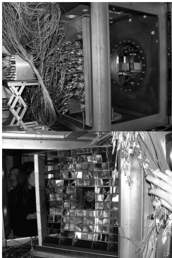
Fig.1 Photo of the experimental set-up mounted inside the TRASMA scattering chamber. In the upper picture the side view of the HODO-SMALL, the back of the HODO-BIG and the targets can be seen. The lower picture shows a front view of the HODO-BIG detector.
