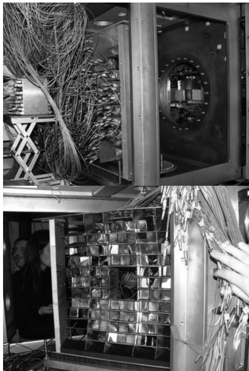
Figure 4: Top: the Hodo-Small (81 two-fold telescopes) back side; bottom: the HODO-Big (89 three-fold telescopes).
