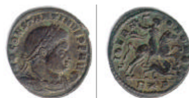
Fig. 1 – The silvered roman coin analysed by means of the non destructive PIXE and XRF techniques. The obverse side (on the left) has been labeled Mon1 during the measurement, while the reverse one (on the right) has been labeled Mon2.
