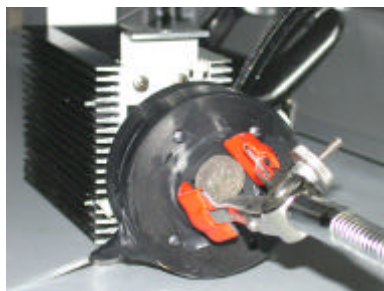
Fig. 4 - The portable PIXE- \alpha system during the measurement of a silvered roman coin. The ^{210}\text{Po} source
