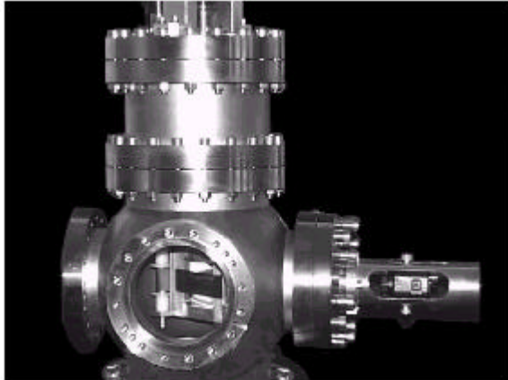
Figure 3: A picture of the LEBI device. The spherical vacuum chamber containing the plate-tape set-up and the germanium detectors will be installed along the beam pipe
