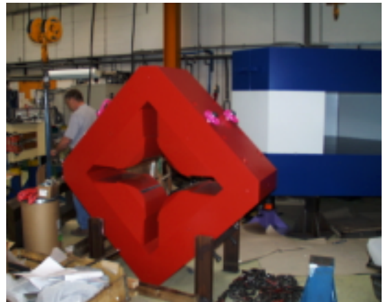
Fig. 1 Photograph of quadrupole (foreground) and dipole (background) yokes at DANFYSIK A/S.
