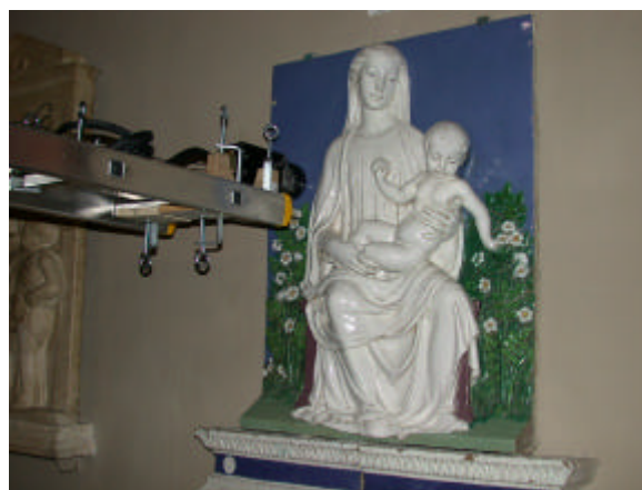
Fig. 6 – The portable PIXE-alpha system during the characterization of a Della Robbia artifact at the Bargello Museum of Florence (Italy).
