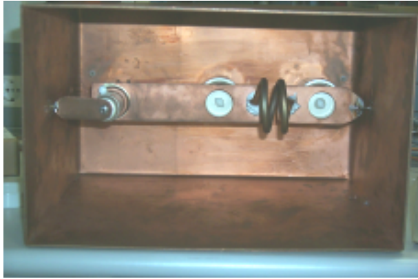
Fig.3: The inner view of the matching box, with the inductance L and the three capacitors C_1 , C_2 and C_3
