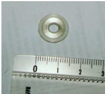
Fig. 2 – The mylar support of the ^{210}\text{Po} source. The annular evaporation of silver is visible on the picture
