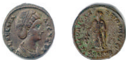
Fig. 3 – The silvered roman coin analysed by means of the non destructive PIXE and XRF techniques. The obverse (on the left) has been labelled GARRA2 during the measurements, while the reverse one (on the right) has been labelled GARRA1.
