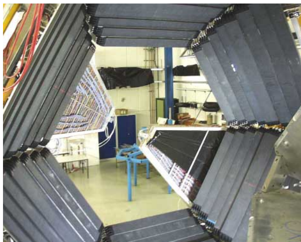
Fig.2 The Time Of Flight wall right after its installation on the HADES mechanical support frame.
