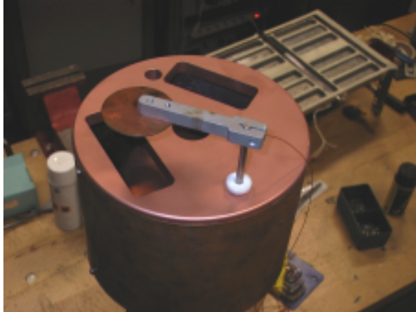
Fig.6: The covered axial buncher before the insertion inside the cyclotron. Clearly visible is the current beam probe which intercepts the beam when placed directly over the central hole. Other apertures have been made to improve the vacuum level inside the buncher.
