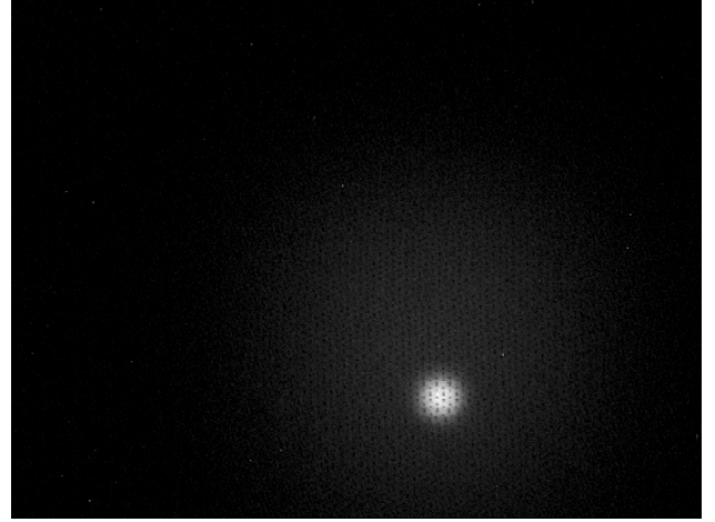
Fig.3 – Live picture of a 30pA proton beam after the 1mm collimator and the lithographic mask while selecting a 150 \mu\text{m} aperture.
