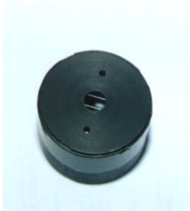
Fig. 2 – The ^{210}\text{Po} source
