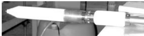
Fig. 5 : new deflector electrical feedthrough in glazed alumina
