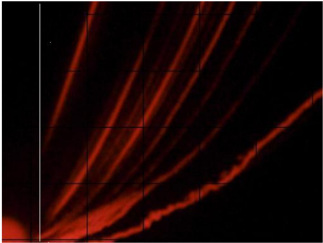
Figure 2.4: Spectrogram in experiment at PALS laboratory showing that each parabolas begin with a line of constant energy per charge (white)
