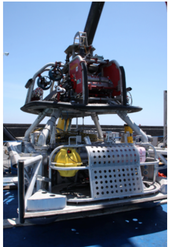
The NEMO-SN1 Observatory on board of the cableship Certamen (owned by Elettra Tlc SpA) before the deployment
