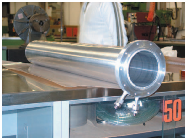
Fig.3- The new aluminum chamber of SERSE over the test bench
