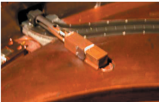
Figure 6: Cooled internal beam current probe
