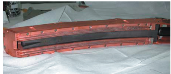
Figure 8: Front part of the new deflector with cooling
