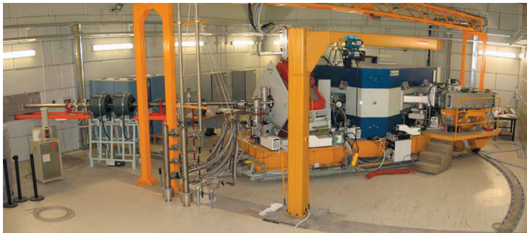
Fig. 1. View from the top of the shielding walls of MAGNEX with the recently-installed FPD on the right. The beam will come from roughly the top-left of the picture.
