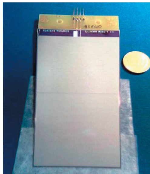
Fig.1 - CHIMERA silicon detector from one telescope of ring 7.
