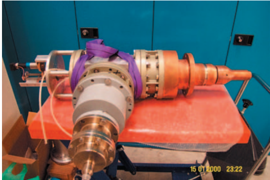
Fig. 7- Coupler for chopper 500
