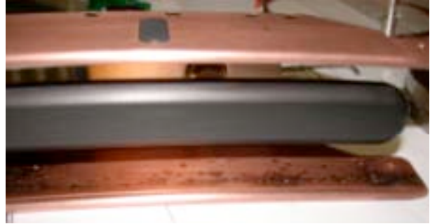
Fig.4- New aluminum electrode hard-anodized
