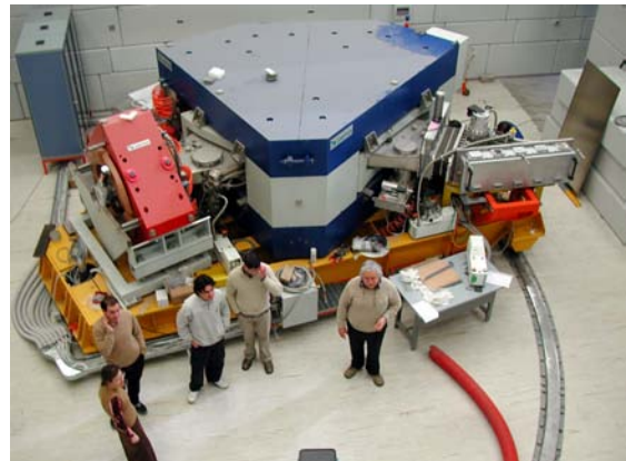
Fig. 1. View from the top of the shielding walls of MAGNEX with the recently-installed FPD on the right. The beam will come from roughly the top-left of the picture.
