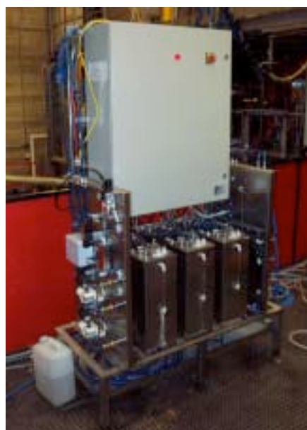
Fig. 13-Cooling rack for diagnostic devices
