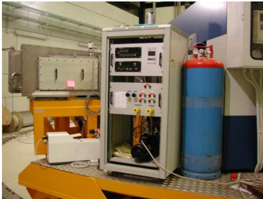
Fig. 3. The gas handling system for the FPD installed on the platform. An access port at the exit of the spectrometer (before the bellows) is seen on the left.
