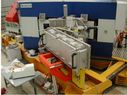
Fig. 2. The FPD box installed at the exit of the spectrometer on the support that allows it to be rolled back for maintenance.
