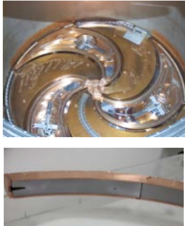
Figure 3: Septum of the electrostatic deflector with damages due to the high beam power
