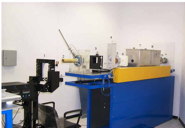
Figure 1. View of the CATANA beam line: 1. Treatment chair for patient immobilization, 2. Final collimator, 3. Positioning laser, 4. Light field simulator; 5. A Monitor chamber; 6. Intermediate collimator, 7-8. Boxes for the location of modulator wheel and range shifter, 9. Proton beam output window.
