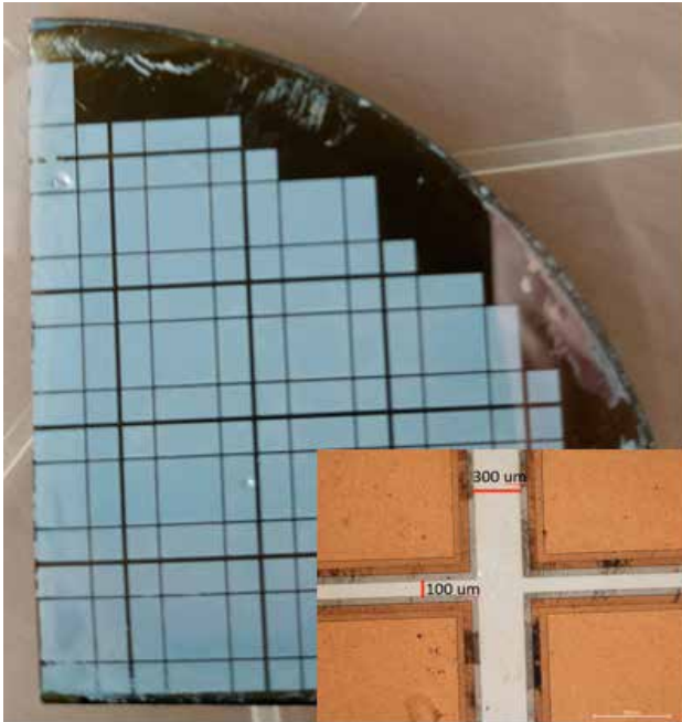
Figure 3. The figure shows the detectors fabricated on SiC epi-layer. On the right there is a magnification carried out with a 5x objective.
