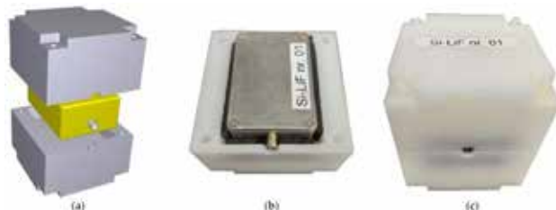
Figure 2: (a) 3D sketch of the SiLiF detector; (b) a SiLiF hosted in a half moderator; (c) final assembling of a SiLiF.
