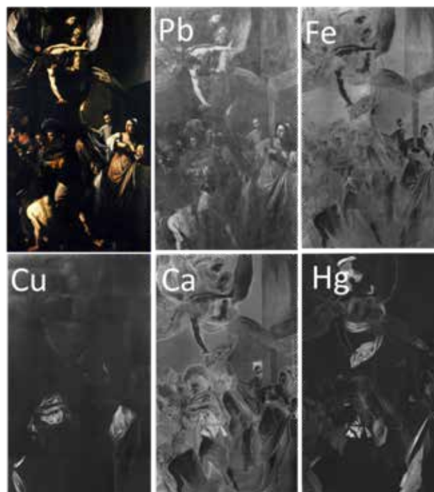
Figure 2: maps of the main chemical elements (Pb, Fe, Cu, Ca, Hg) characterizing the pigments used by Caravaggio for painting "Seven Works of Mercy".
