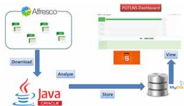
Figure 2 - Details of the system architecture
