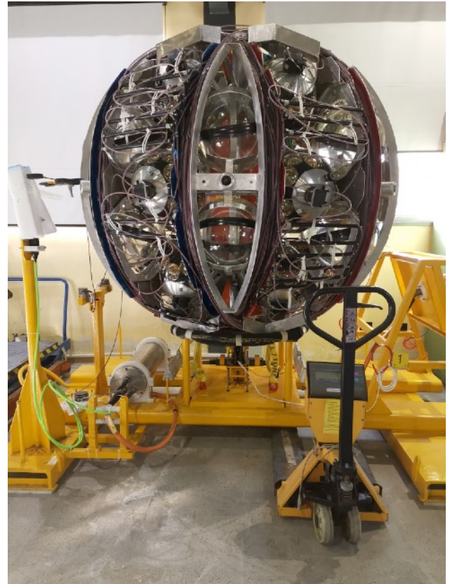
Figure 3: ARCA DU fully integrated before deployment
