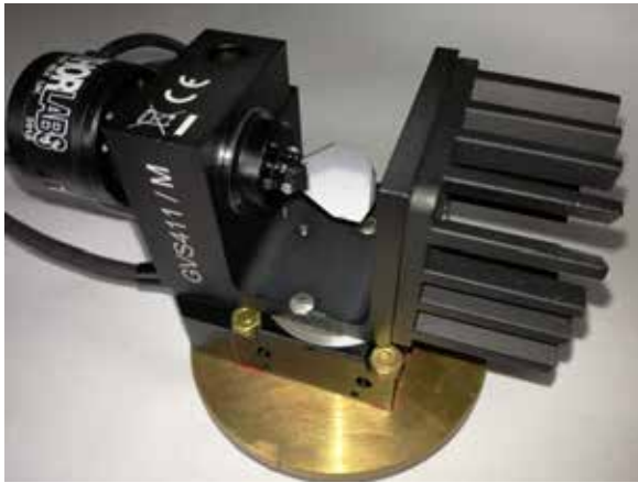
Figure 2: Galvo system and rotation stage used for the rotation of the mirror around two orthogonal axes.
